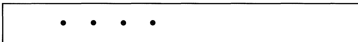
Example 4: Four 1/16 in. (1.6 mm) discontinuities
